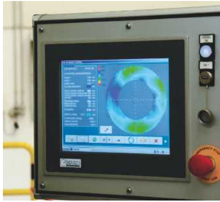
A laser reads to blade surface indicating any minute anomalies, shown up on screen as a different colour
